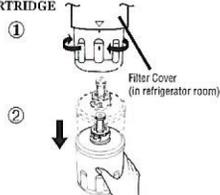
**2** Apply the month sticker to the cartridge as a reminder to replace the filter within 6 months and remove red cap.
