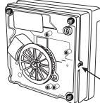
To remove cover, pull straight forward. When facing the level adjustment screw make a 1/2 turn clockwise to decrease the water flow by 20 cc's. Turning counter-clockwise to increase water flow.
